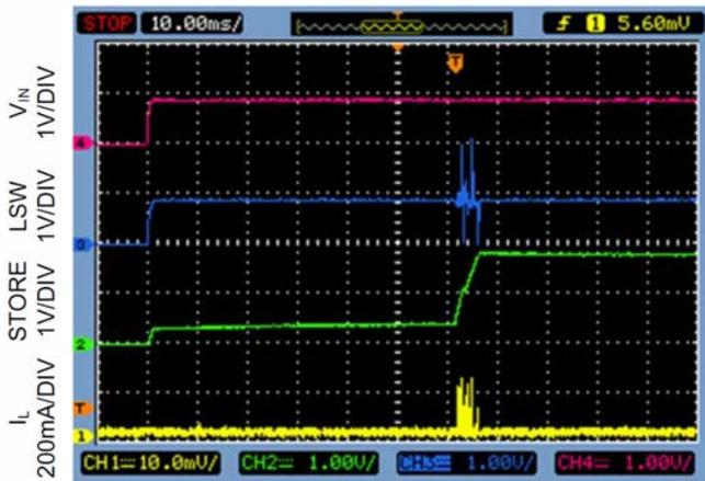
Startup : Circuit A with  $R_{IN}=10\Omega$
