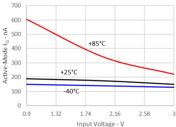
Active-Mode  $I_Q$  vs Input Voltage
