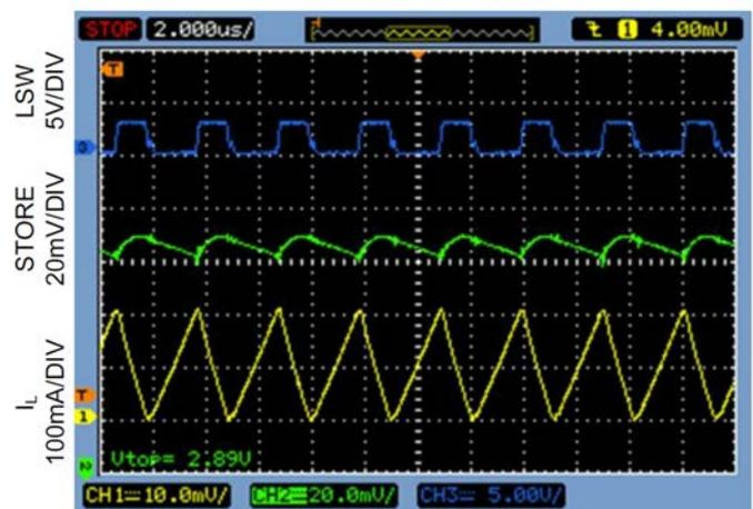
Startup : Circuit A with  $R_{IN}=10\Omega$
