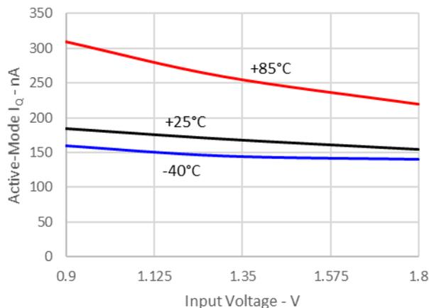
Active-Mode  $I_Q$  vs Input Voltage
