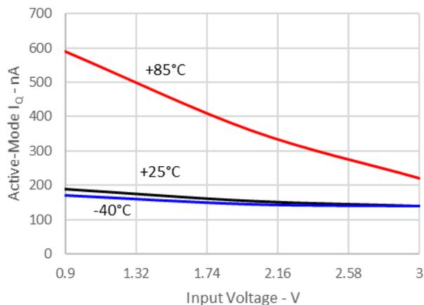
Active-Mode  $I_Q$  vs Input Voltage
