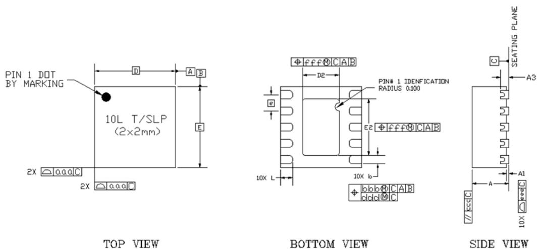
Figure 5.1. TS3310/12/14 2x2 mm 10-QFN Package Diagram
