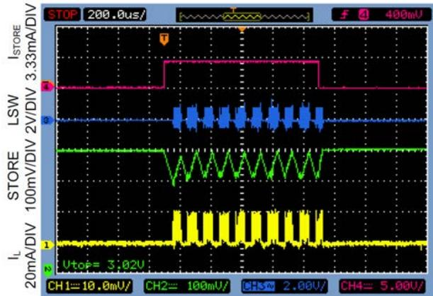
STORE Output Voltage Ripple, Inductor Current, and LSW Voltage : Circuit A
