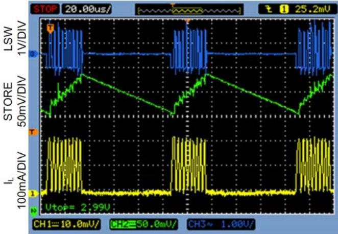
STORE Output Voltage Ripple, Inductor Current, and LSW Voltage : Circuit A
