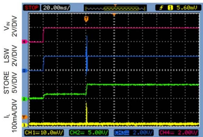
Startup : Circuit A with  $R_{IN}=10\Omega$
