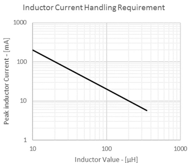
**Figure 2.5. Inductor Peak Current vs. Inductor Value**
