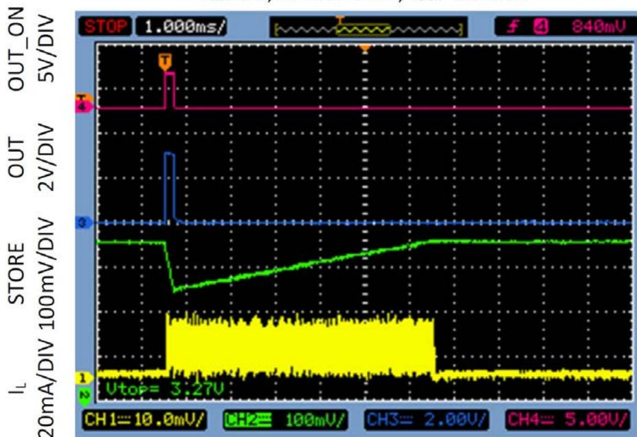
Figure 2.8. 220  $\mu$ F  $C_{STORE}$  Recovery Scope Capture
