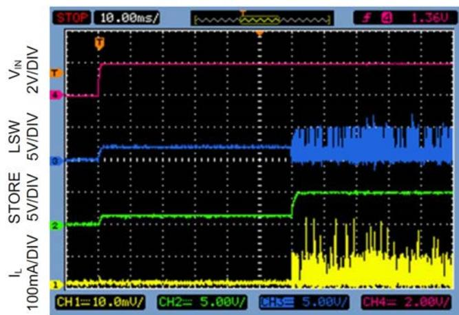
OUT\_ON Switched ON : Circuit A with C<sub>OUT</sub> Removed
