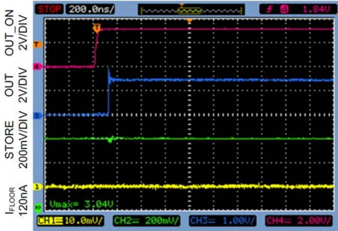
OUT\_ON Switched OFF : Circuit A with C<sub>OUT</sub> Removed
