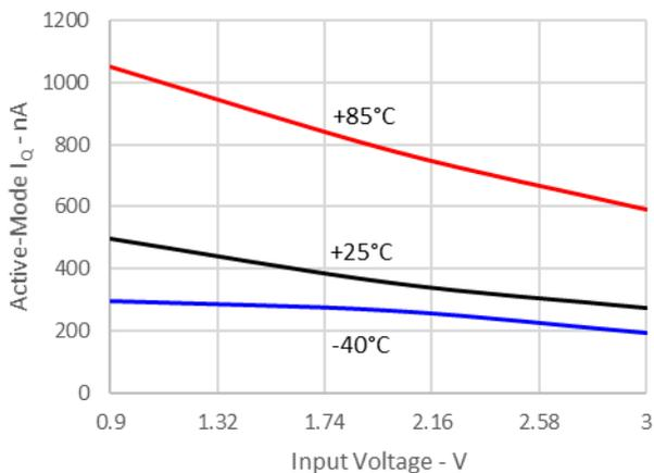
Active-Mode  $I_Q$  vs Input Voltage
