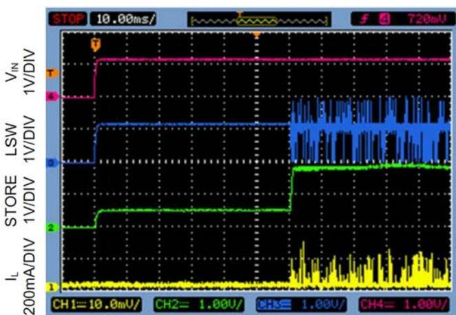
Startup : Circuit A with  $R_{IN}=10\Omega$
