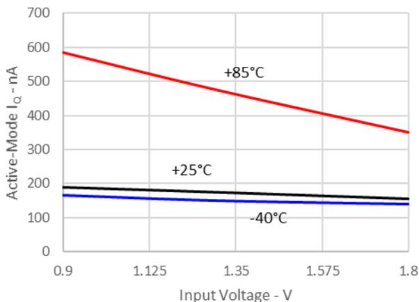
Active-Mode  $I_Q$  vs Input Voltage
