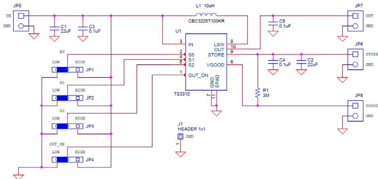
**Figure 2.1. TS331x-EVB Schematic**
