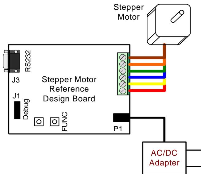
**Figure 2. Stepper Motor Reference Design Demonstration Setup**
