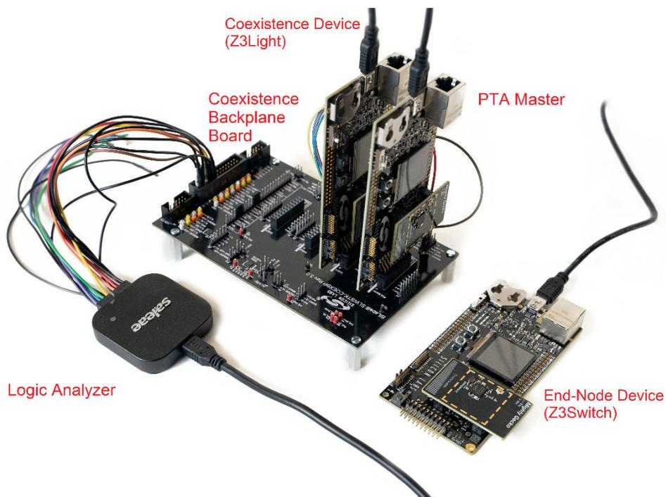
Figure 1.2. Coexistence Test Setup Using a Zigbee Example (1)
