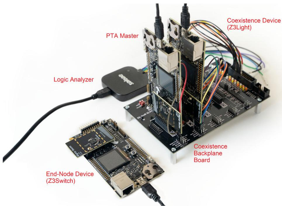
Figure 1.3. Coexistence Test Setup Using a Zigbee Example (2)
