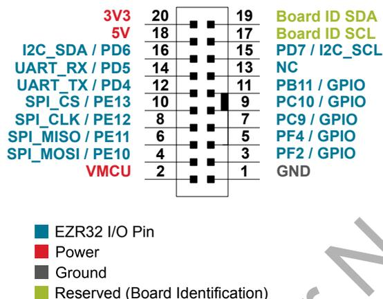
Figure 3.3. Expansion Header
