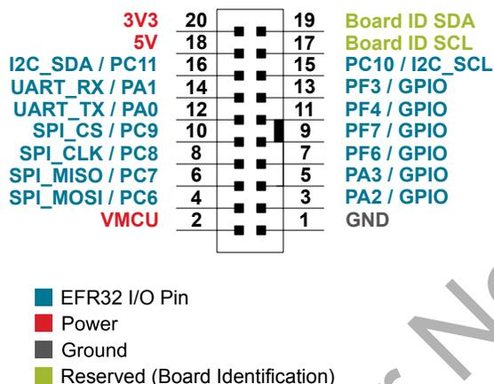
Figure 3.3. Expansion Header
