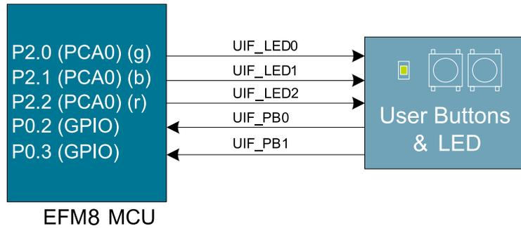
**Figure 5.1. Buttons/LEDs**
