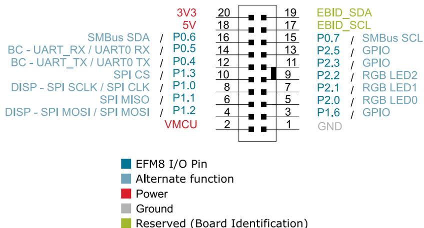
Figure 6.2. Expansion Header
