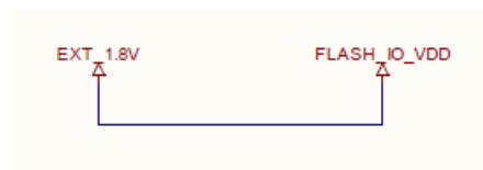
Figure 8.12. Option 2: In-Package PSRAM Powered From External 1.8 V Supply
