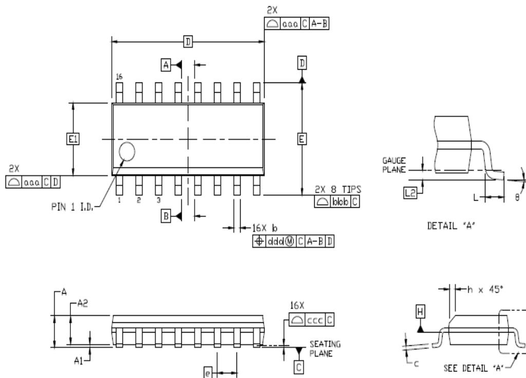
Figure 7.2. 16-pin Small Outline Integrated Circuit (SOIC) Package
