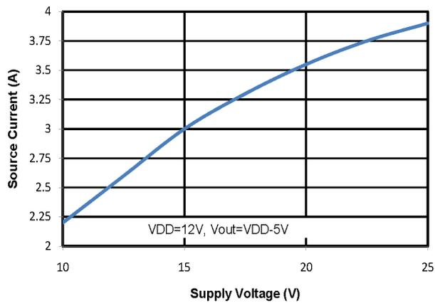
Figure 3.26. Output Source Current vs. Supply Voltage
