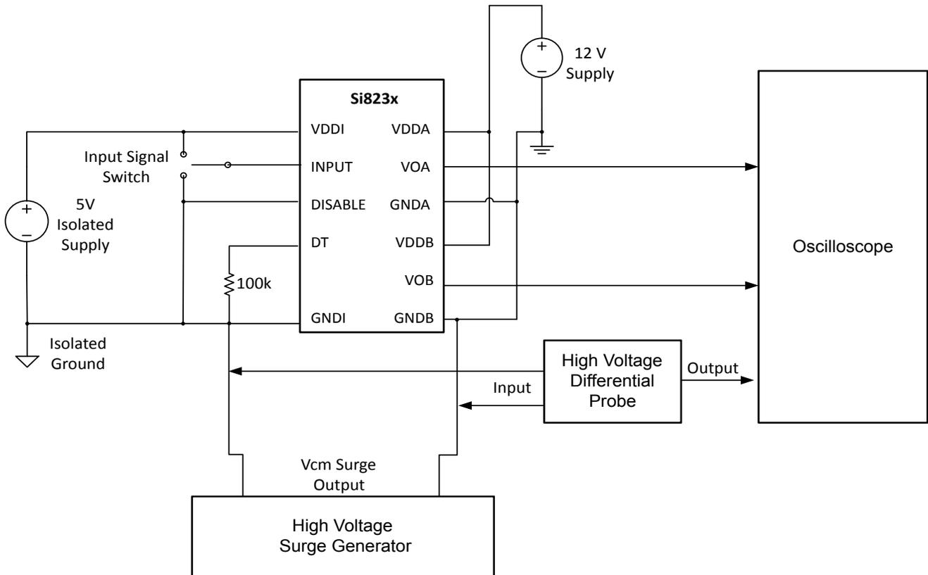
Figure 4.3. Common Mode Transient Immunity Test Circuit
