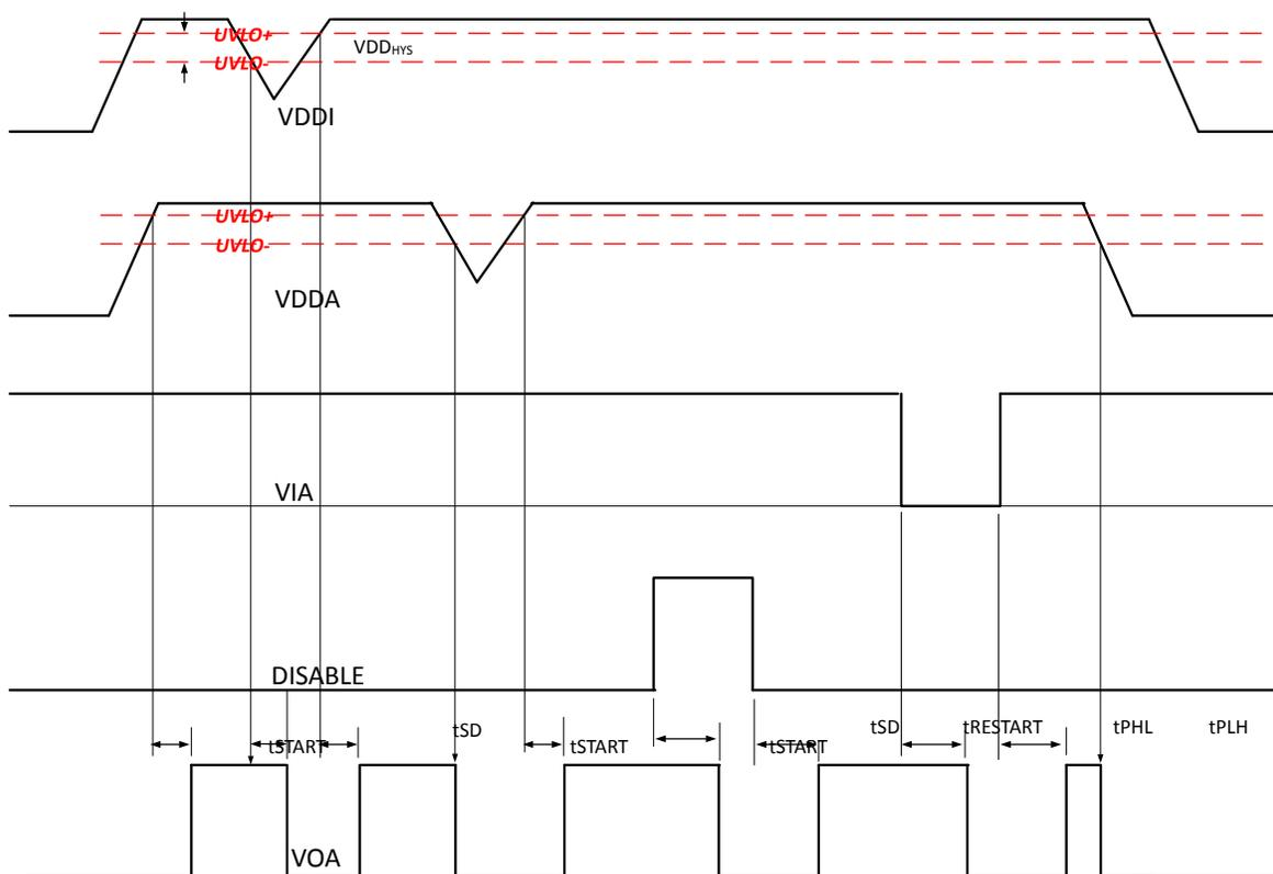
Figure 3.30. Device Behavior during Normal Operation and Shutdown
