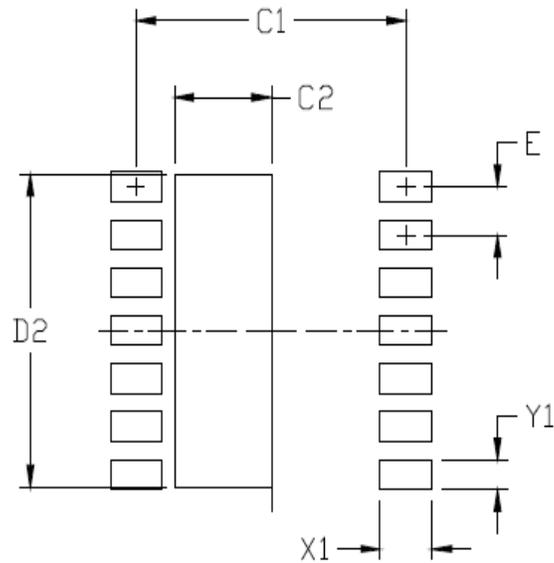
Figure 8.4. 14-Pin LGA with Thermal Pad Land Pattern
