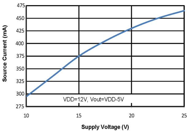
Figure 3.14. Output Source Current vs. Supply Voltage
