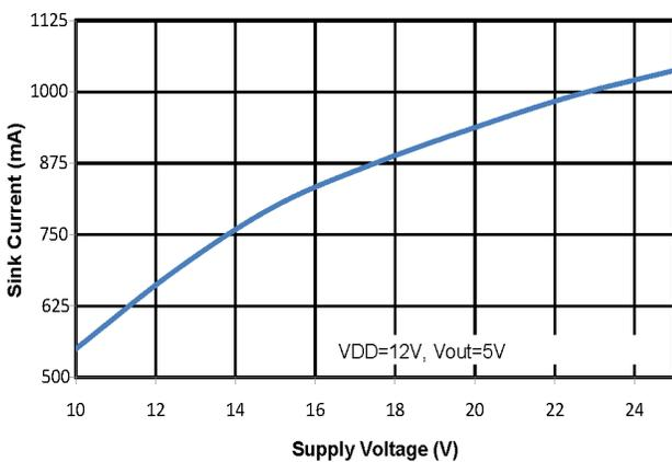
Figure 3.16. Output Sink Current vs. Supply Voltage
