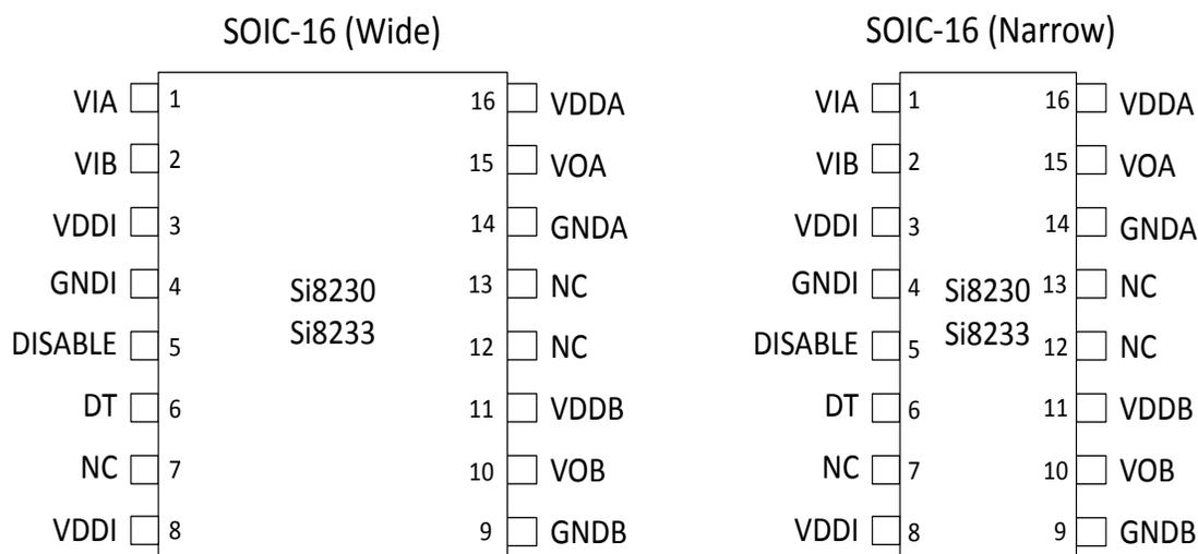
Table 6.1. Si8230/3 Two-Input HS/LS Isolated Driver (SOIC-16)
