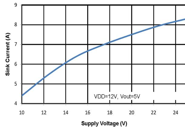
Figure 3.28. Output Sink Current vs. Supply Voltage
