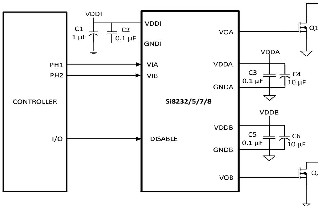
**Figure 5.2. Si8232/5/7/8 in a Dual Driver Application**
