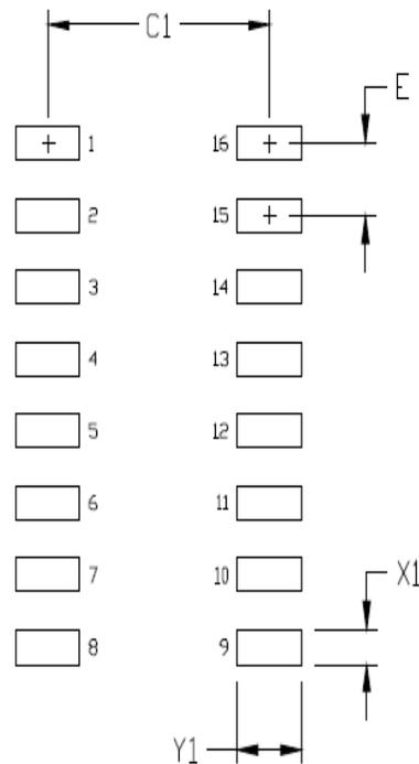
Figure 8.2. 16-Pin Narrow Body SOIC PCB Land Pattern
