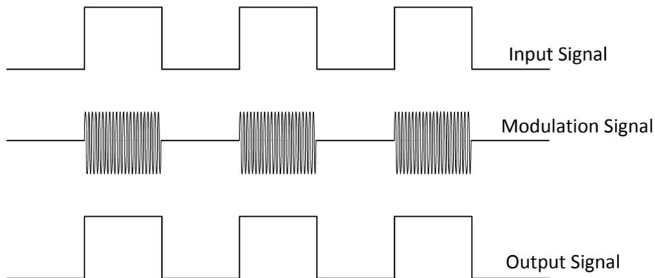
Figure 3.5. Modulation Scheme
