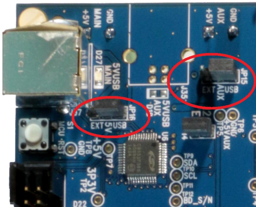
**Figure 9.2. JP15-JP16 Standard Jumper Shunt Installation**
