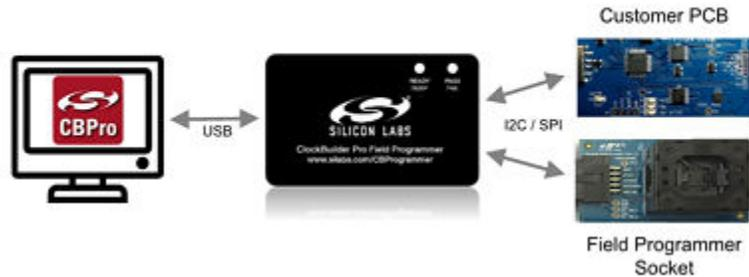
Figure 4.1. PC to CBPROG-DONGLE Connection
