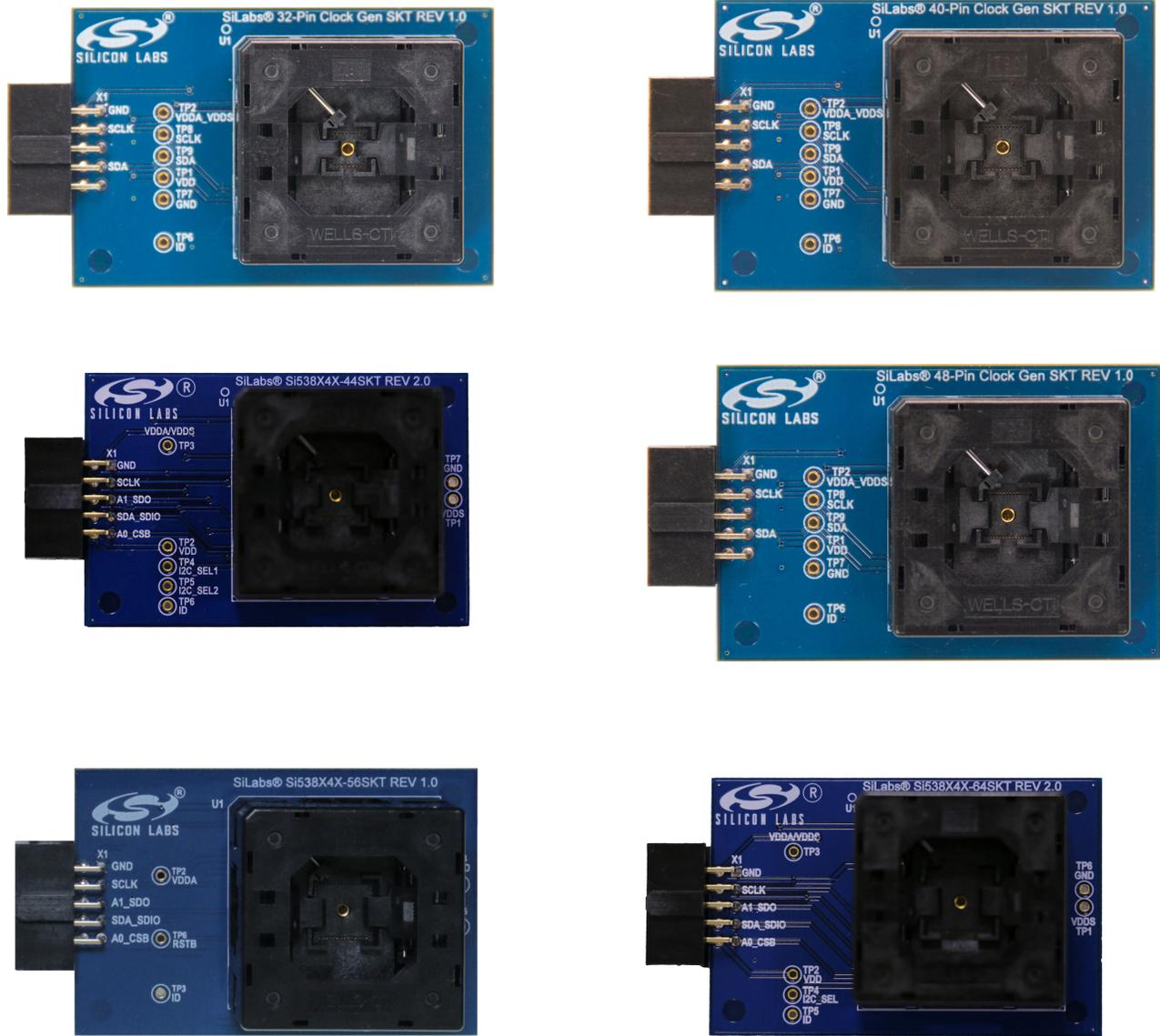
**Figure 1.3. Si5332-32SKT-DK, Si5332-40SKT-DK, Si538x4x-44SKT-DK, Si5332-48SKT-DK, Si538x4x-56SKT-DK, Si538x4x-64SKT-DK Sockets Sold Separately**
