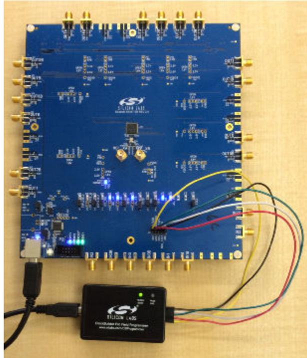
**Figure 4.16. Example I<sup>2</sup>C Connection to External System Target Board Using Jumper Wires (Si5346-EVB)**
