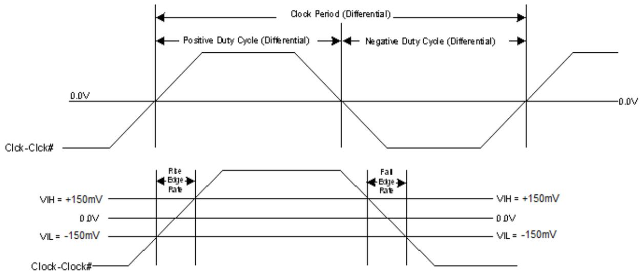
**Figure 2. Differential Output Signals (for AC Parameters Measurement)**
