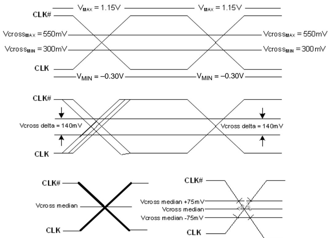
**Figure 3. Single-ended Measurement for Differential Output Signals
