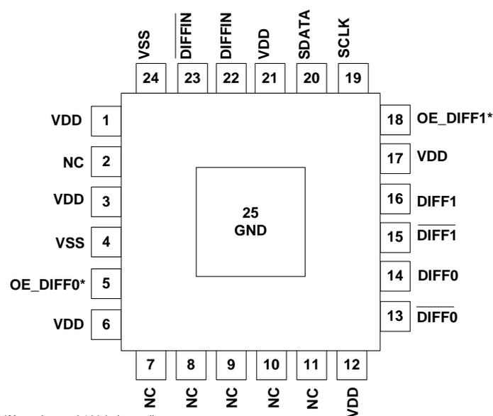
Figure 4. 24-Pin QFN
