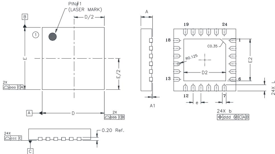
**Figure 5. 24-Pin Quad Flat No Lead (QFN) Package**
