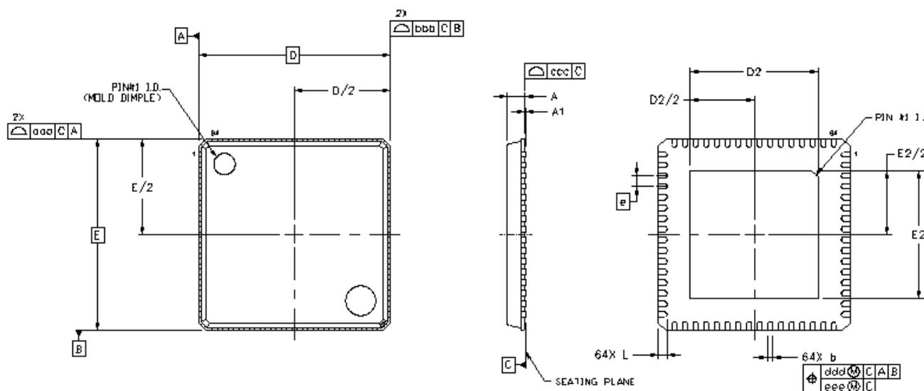
Figure 12. 64-Pin Quad Flat No Lead (QFN) Package
