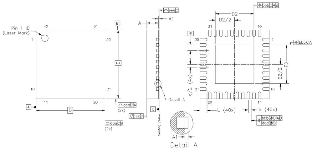
**Figure 12. 40-Pin Quad Flat No Lead (QFN) Package**
