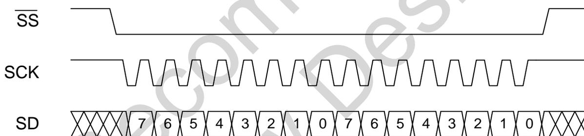
Figure 7. SPI-Like Interface Write/Set Address Command
