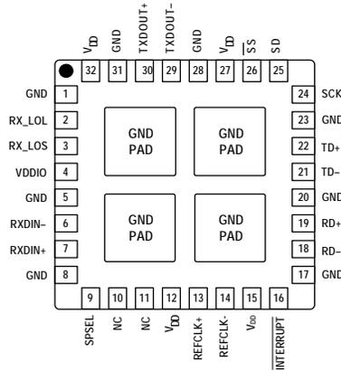
Figure 24. Si5040 Pin Configuration (Transparent Top View)
