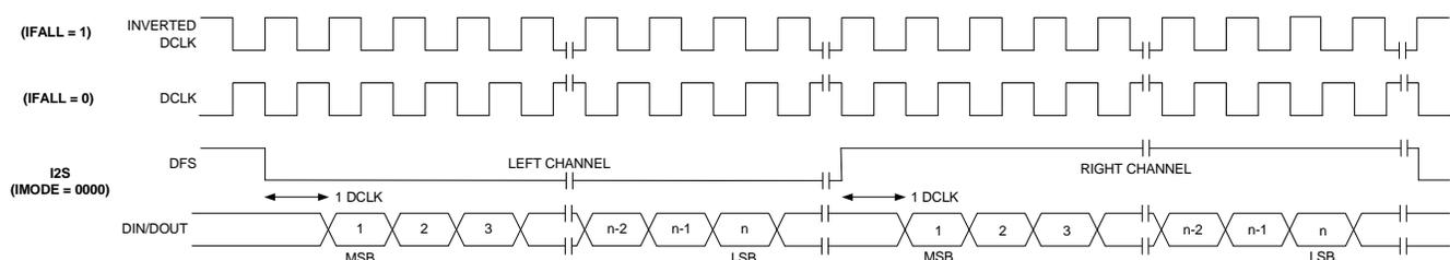
Figure 21. I<sup>2</sup>S Digital Audio Format
