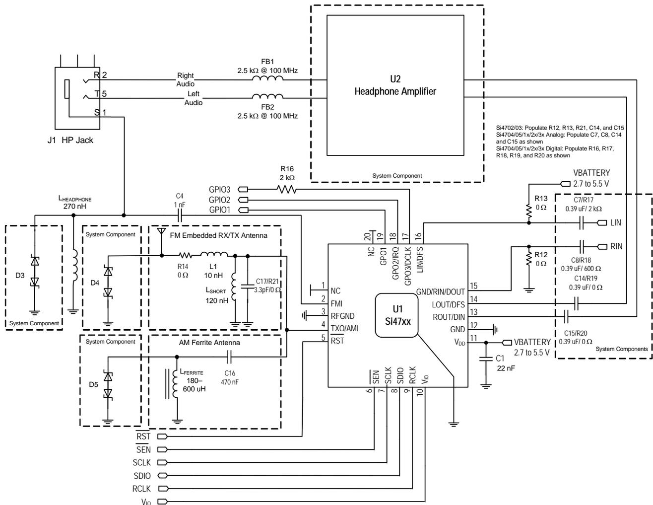
**Figure 13. Universal AM/FM RX/FM TX Application Schematic**
