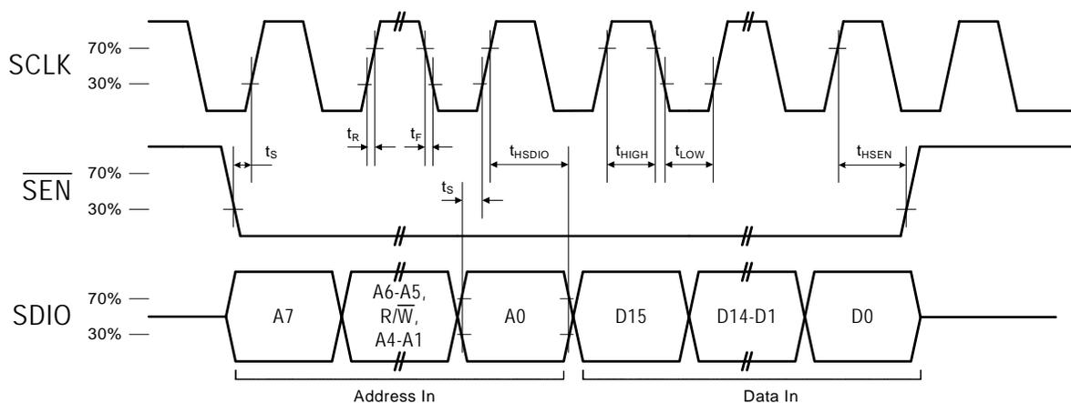
**Figure 4. 3-Wire Control Interface Write Timing Parameters**
