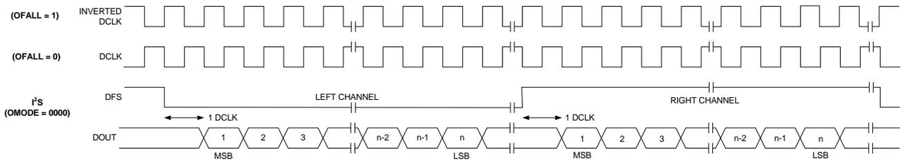
**Figure 16. I<sup>2</sup>S Digital Audio Format**
