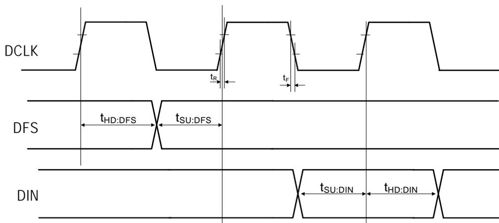
**Figure 9. Digital Audio Interface Timing Parameters, I<sup>2</sup>S Mode**
