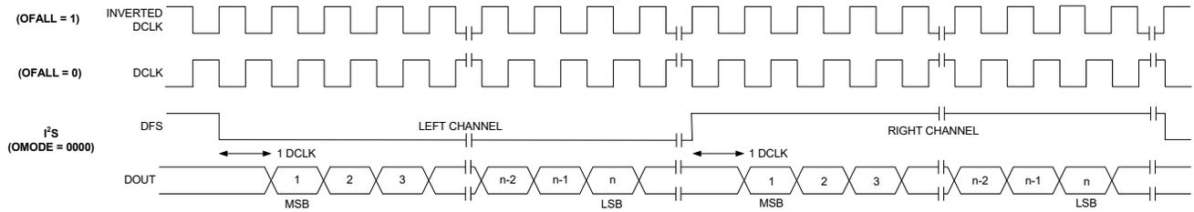
Figure 9. I<sup>2</sup>S Digital Audio Format
