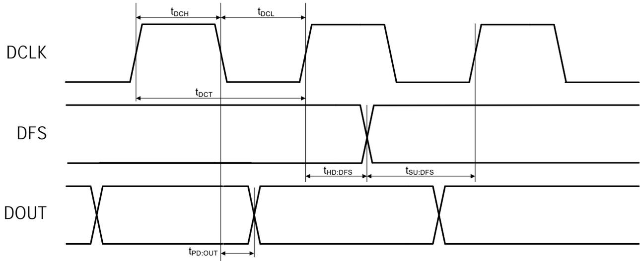
**Figure 6. Digital Audio Interface Timing Parameters, I²S Mode**
