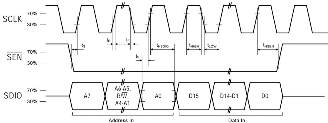
**Figure 4. 3-Wire Control Interface Write Timing Parameters**
