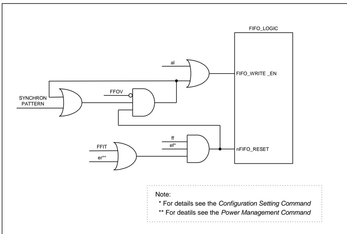
Bit 1 ( $ff$ ): FIFO fill will be enabled after synchron pattern reception. The FIFO fill stops when this bit is cleared.
