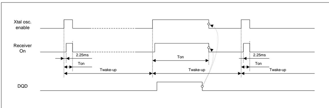
Bit 0 (en): Enables the Low Duty-Cycle Mode. Wake-up timer interrupt not generated in this mode.
