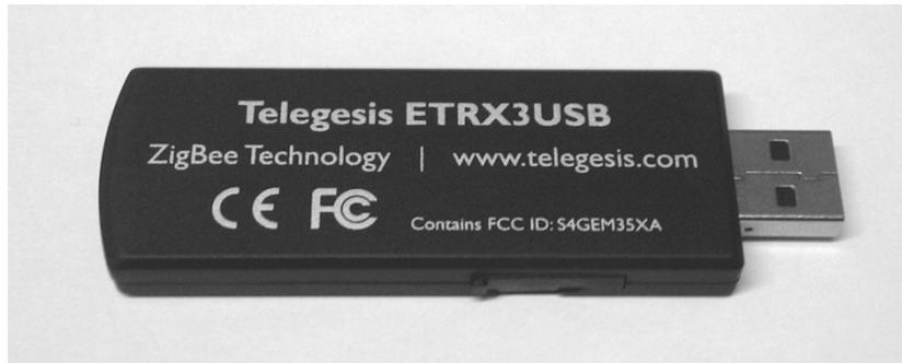
The ETRX3USB ZigBee USB Stick is effectively an RS232 to USB bridge connected to an ETRX3 Series ZigBee module. This allows connectivity to a computer's USB port.
