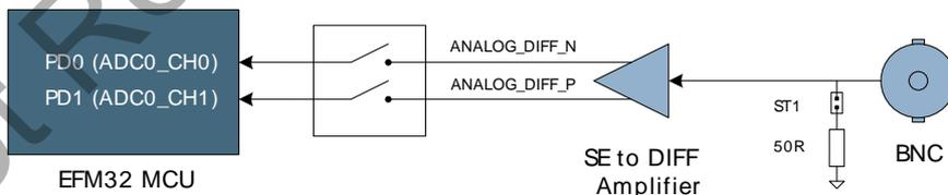
This peripheral can be connected by calling:
