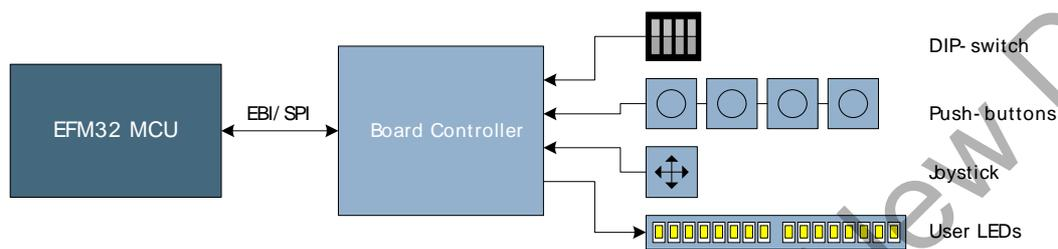
The buttons and LEDs are not directly connected to the MCU, instead the board controller is used to read button states and set the LED outputs. This can be done with a set of BSP API functions
