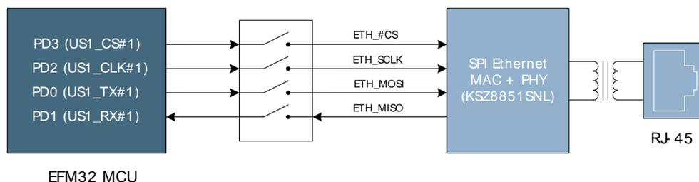
The Ethernet controller has 12KB buffer memory on the receive queue and 6KB on the transmit queue, and supports Auto-MDIX. Two LEDs are placed next to the RJ-45 connector to indicate link speed and activity.
