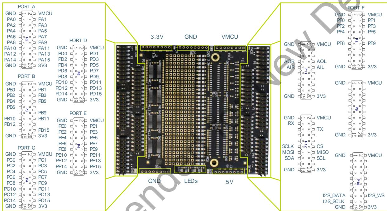
Additionally, the Prototyping Board also contains connection points for different voltages: 3.3V, 5V, GND, and VMCU. Any current drawn from the VMCU pins will also be measurable with the Advanced Energy Monitor, allowing the whole circuit to be evaluated.
