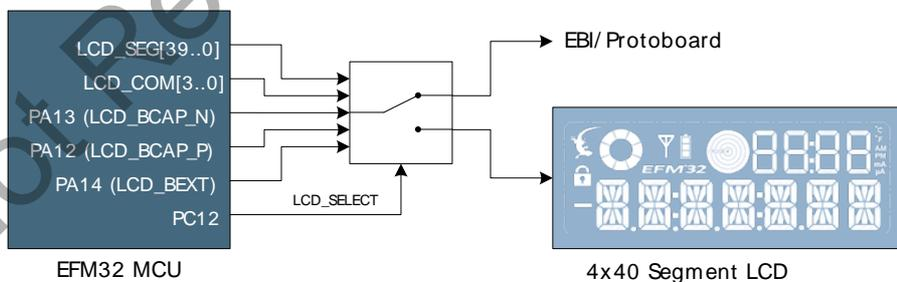
When the LCD\_SELECT signal is enabled, a 22nF capacitor is connected between LCD\_BCAP\_N and LCD\_BCAP\_P, and a 1uF capacitor is connected between LCD\_BEXT and GND. This allows the use of the internal voltage booster to power the LCD if desired.
