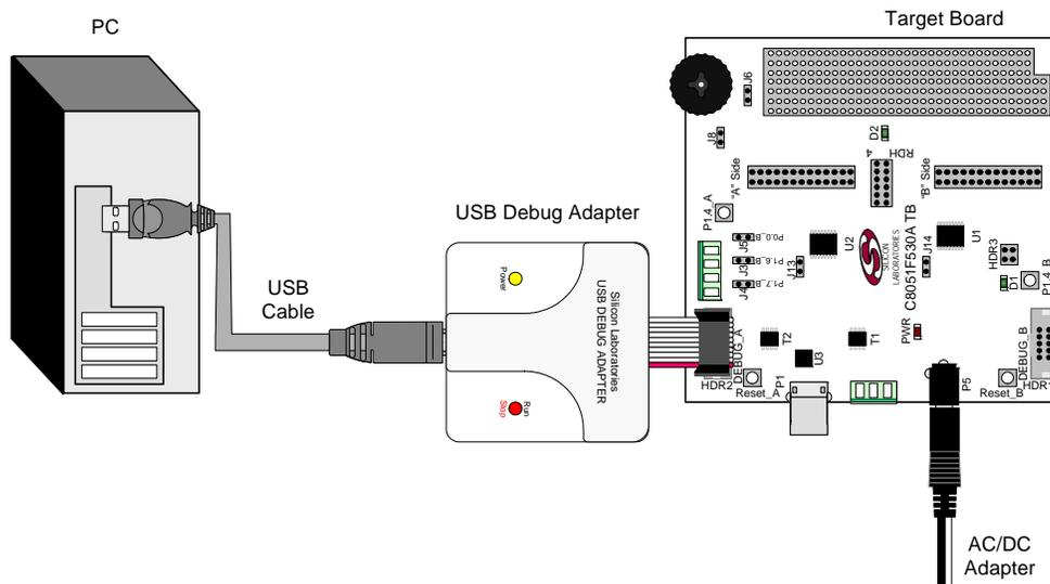
Figure 1. Hardware Setup using a USB Debug Adapter
