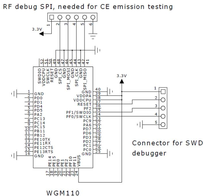
**Figure 3.6. SWD Debug and RF Test Interface Connections**
