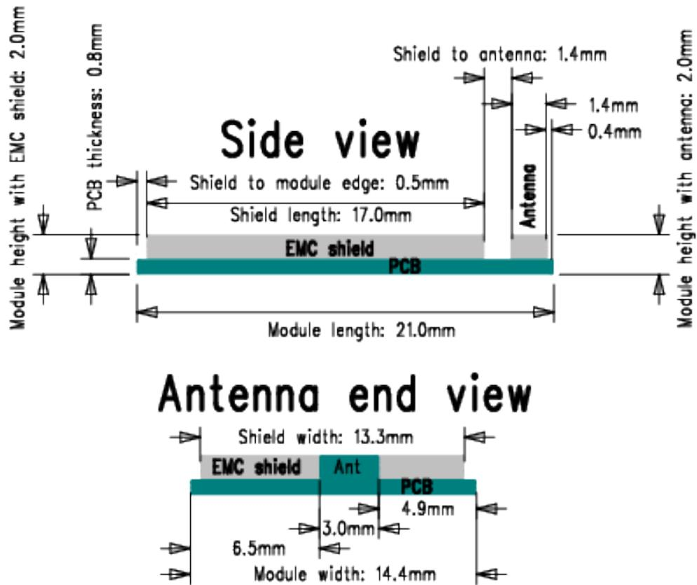
Figure 8.2. Side and Antenna End View Dimensions (WGM110A)
