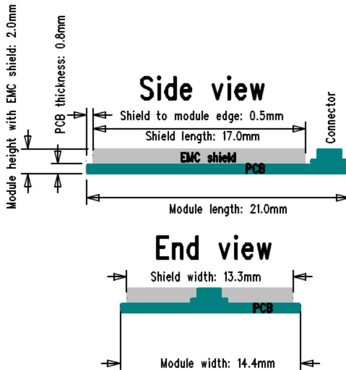
**Tolerance  $\pm 0.1\text{mm}$  for all measurements**
