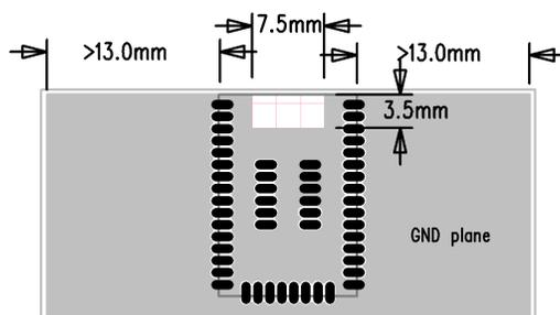
Figure 5.1. Recommended Application PCB Layout for WGM110A Module
