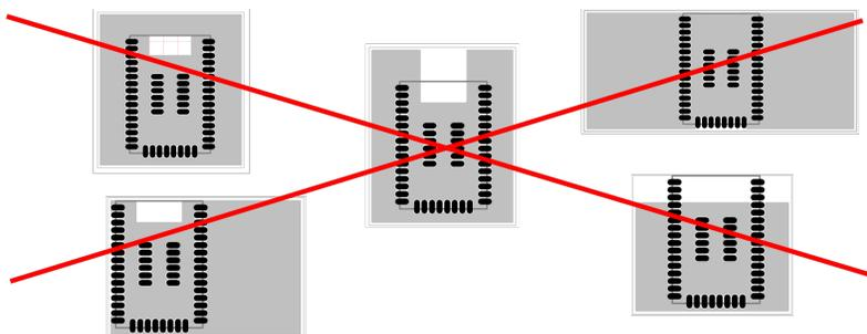
**Figure 5.2. Non-optimal Application PCB Layouts for WGM110A Module**
