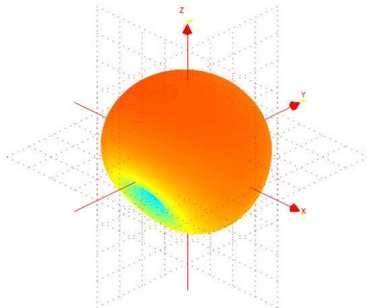
Figure 7.1. Typical 3D Radiation Pattern for WGM110A Module
