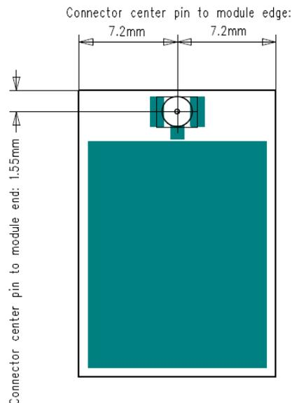
Figure 8.4. u.FL Connector Placement on the WGM110E Module
