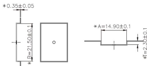
Figure 10.2. Dimensions of the Module Slot on Tape
