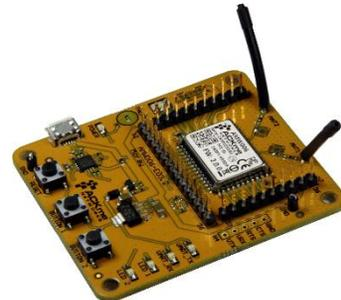
Figure 10 - AMW006-E03 eval board with wire antennas
