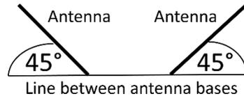
**NOTE!** Do NOT bend antennas backwards over the module; doing so will cause poor performance and may cause undesirable out-of-band radio transmissions.
