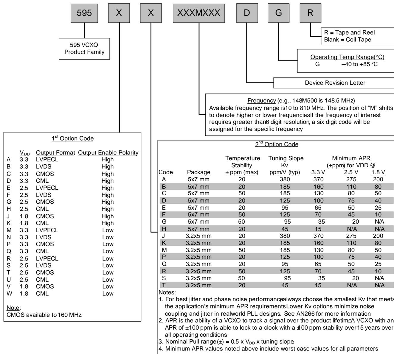
Example Part Number. 595AE148M500DGR is a 5 x 7 mm VCXO in a 6 pad package. The nominal frequency is 148.5 MHz, with a 3.3 V supply, LVPECL output, and Output Enable active high polarity. Temperature stability is specified as  $\pm 20$  ppm and the tuning slope is 95 ppm/V. The part is specified for a -40 to +85 °C ambient temperature range operation and is shipped in tape and reel format.
