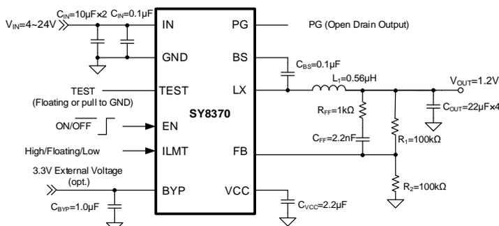
Figure1. Schematic Diagram
