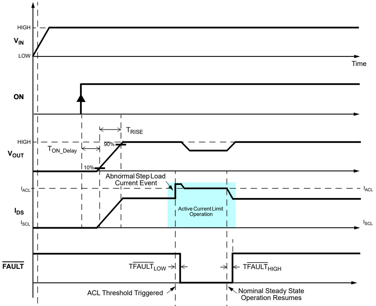
Timing Diagram - Active Current Limit & Thermal Protection Operation
