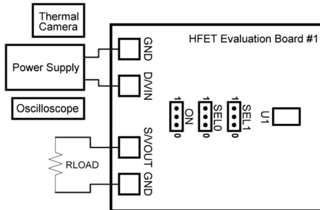
Figure 16. SLG59H1010V Evaluation Board Connection Circuit
