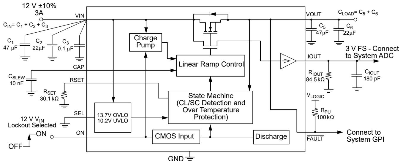
A 13.3 mΩ, 5 A Integrated Power Switch with 12 V / 24 V V<sub>IN</sub> Lockout Select and MOSFET Current Monitor Output
