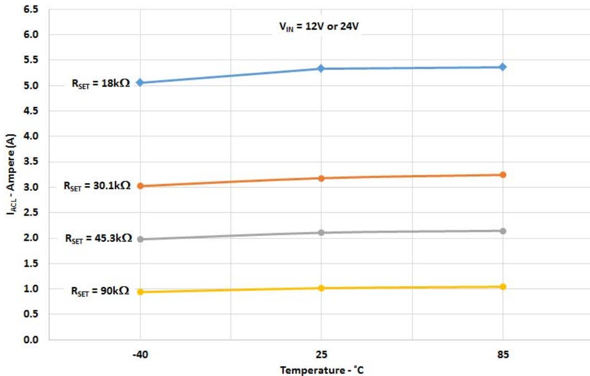
A 13.3 mΩ, 5 A Integrated Power Switch with 12 V / 24 V  $V_{IN}$  Lockout Select and MOSFET Current Monitor Output
