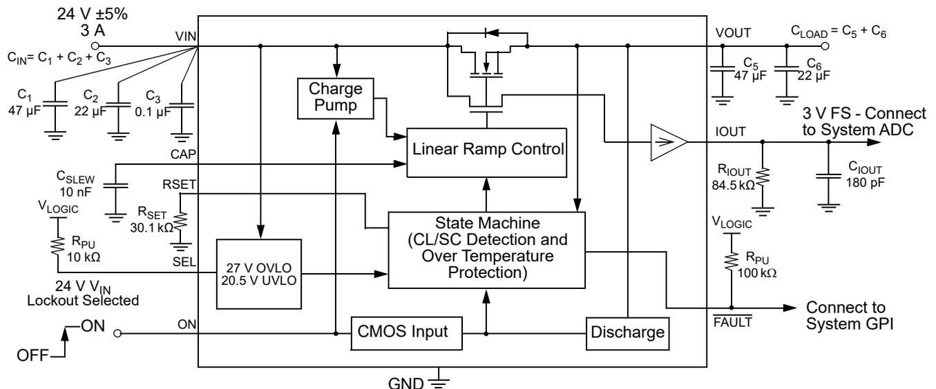
A 13.3 mΩ, 5 A Integrated Power Switch with 12 V / 24 V  $V_{IN}$  Lockout Select and MOSFET Current Monitor Output
