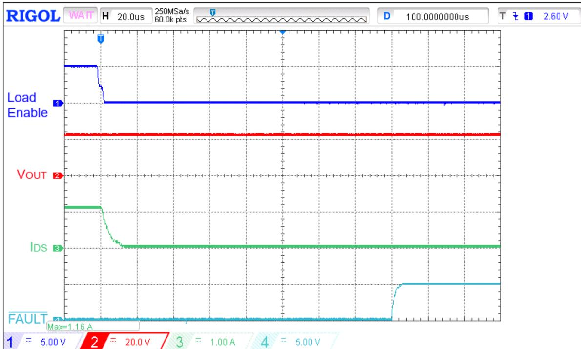
Figure 13. Typical  $\overline{\text{FAULT}}$  de-assertion waveform for  $V_{IN} = 24\text{ V}$ ,  $C_{LOAD} = 10\ \mu\text{F}$ ,  $I_{ACL} = 1\text{ A}$ ,  $R_{SET} = 91\text{ k}\Omega$ , switch out  $18.5\ \Omega$  load
