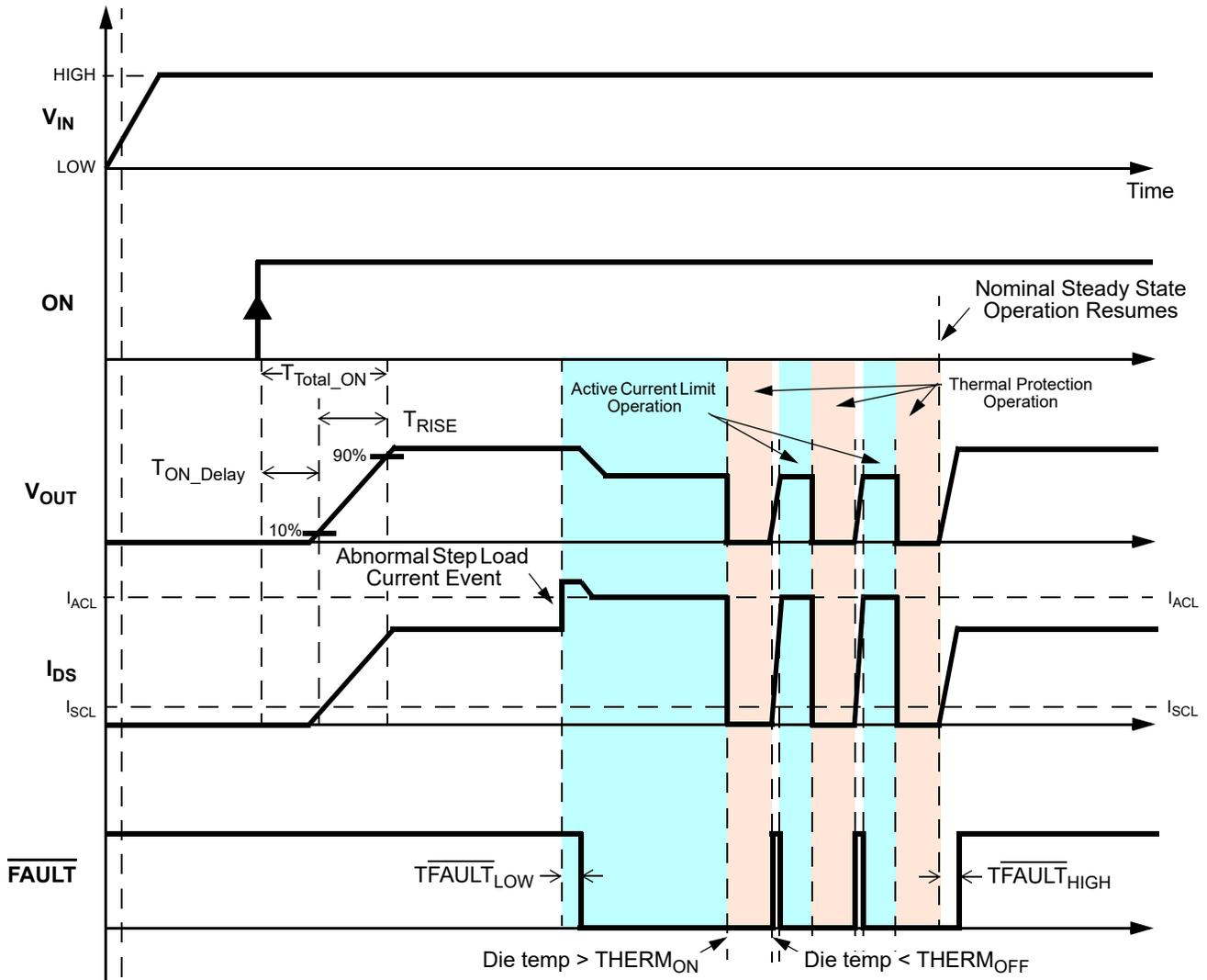
A 13.3 mΩ, 5 A Integrated Power Switch with 12 V / 24 V
