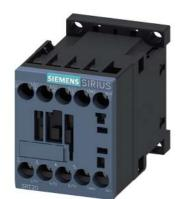
power contactor, AC-3e/AC-3, 9 A, 4 kW / 400 V, 3-pole, 24 V DC, 0.85-1.85\* Us, with integrated diode, auxiliary contacts: 1 NO, screw terminal, size: S00, not expandable with auxiliary switch
