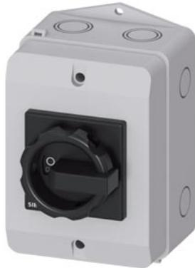
SENTRON, Switch disconnecter 3LD, main switch, 3-pole, Iu: 16 A, Operating power / at AC-23 A at 400 V: 7.5 kW, molded-plastic encapsulation for inch cable gland, rotary operating mechanism, black
