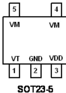
Figure 2. PIN Configuration
