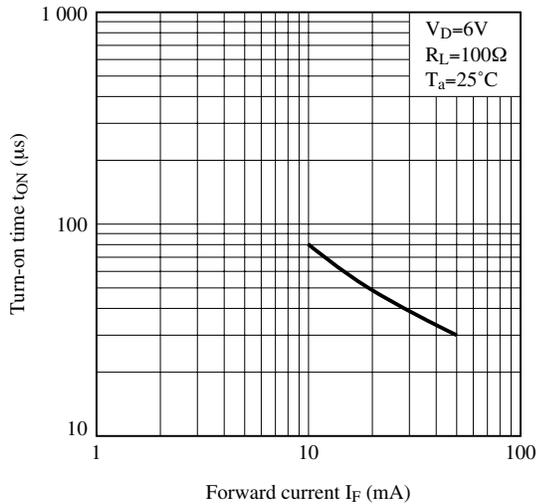
**Fig.10-b Turn-on Time vs. Forward Current (Rank L)**
