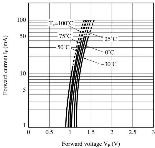
**Fig.3-b Forward Current vs. Forward Voltage (Rank L)**
