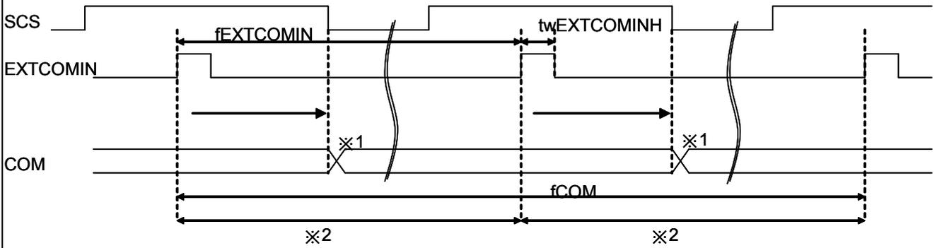
※ 1: LC inversion polarity has been set by the falling edge of SCS signal.
