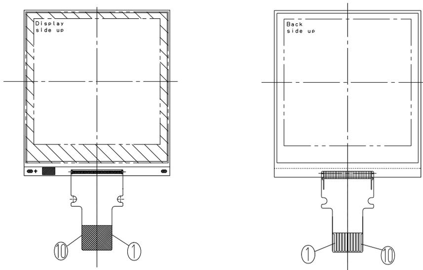
Figure 4-1 Terminals assigned number
