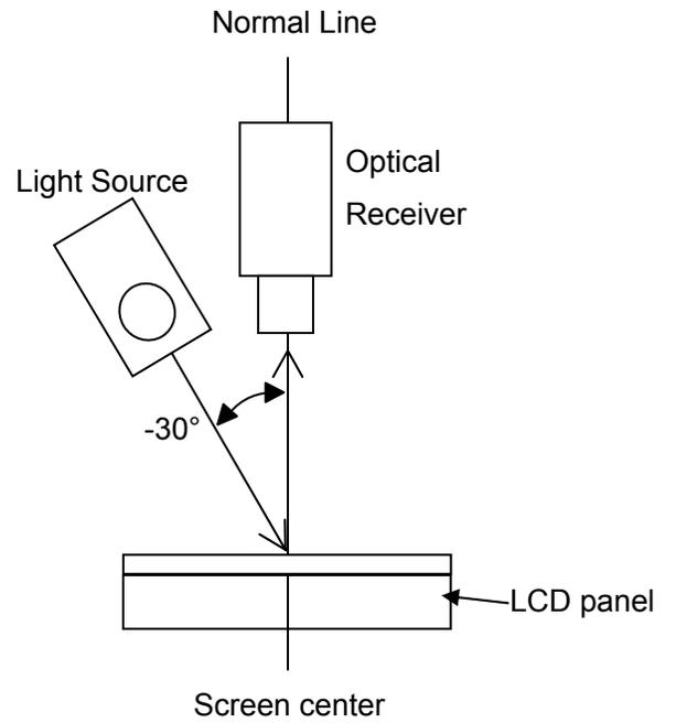
Figure 18 Measurement of contrast, reflective ratio and panel surface chromaticity
