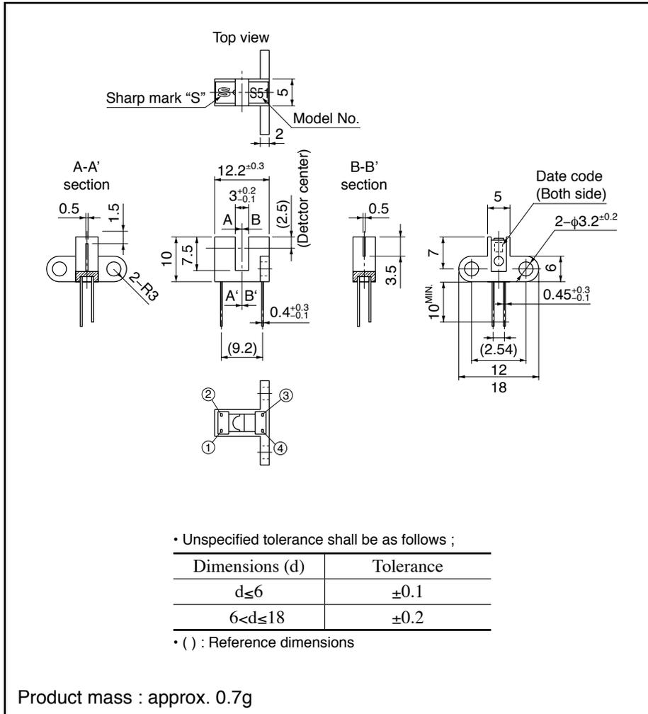
Dip soldering material : Sn-3Ag-0.5Cu
