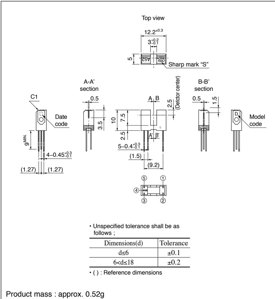
Dip soldering material : Sn-3Ag-0.5Cu
