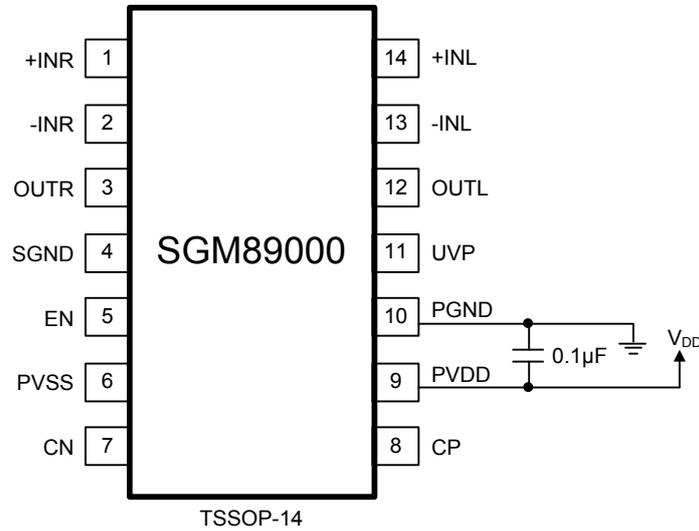
NOTE: 0.1µF decoupling capacitor must be close to PGND and PVDD pins; capacitor can be connected between PVDD and PGND pins directly and then connect PGND pin to GND layer.
