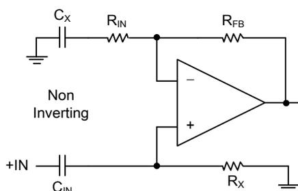
**Figure 3. Non-Inverting**
