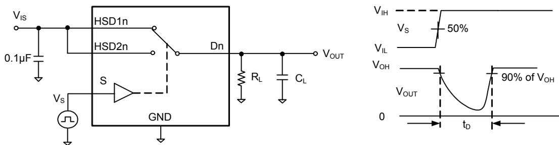
Test Circuit 3. Break-Before-Make Time ( $t_D$ )
