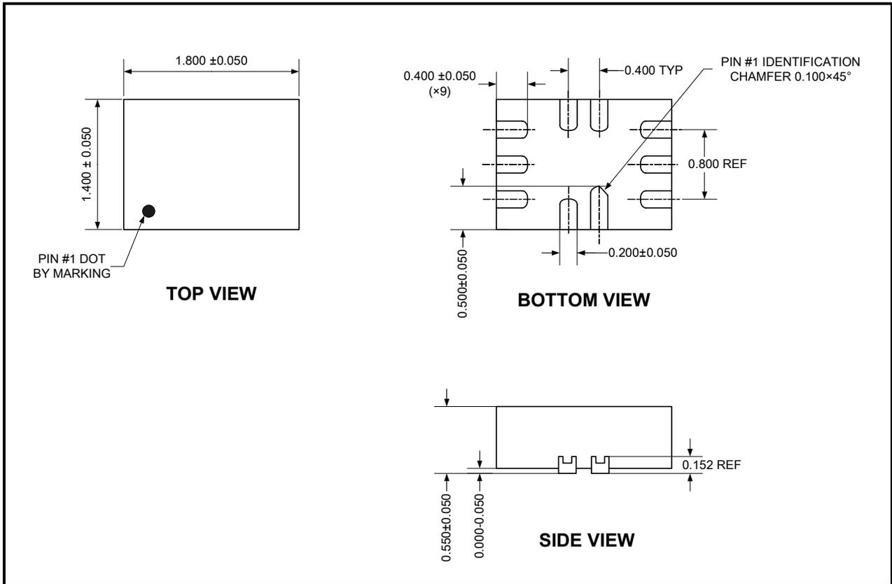
NOTE: All linear dimensions are in millimeters.
