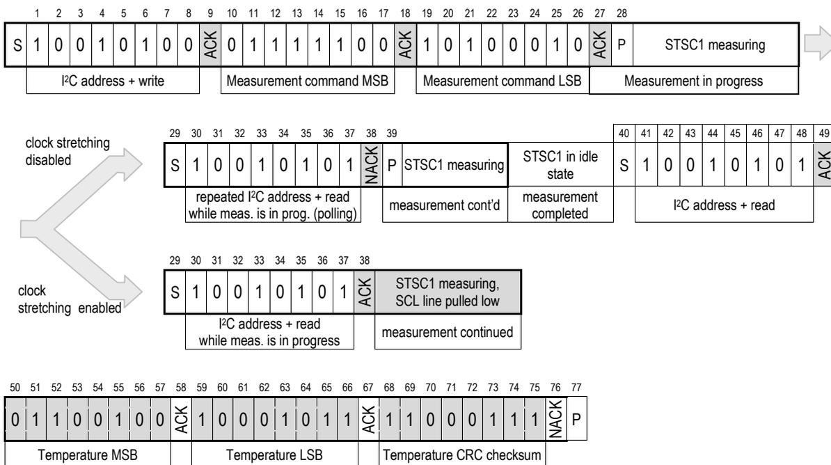
**Figure 5** Communication sequence for starting a measurement and reading measurement results displaying both clock stretching options. The numerical example corresponds to a measurement command with clock stretching enabled. The physical values of the transmitted measurement result is 23.7 °C. Clear blocks are controlled by the microcontroller, grey blocks by the STSC1.
