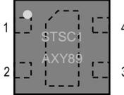
**Table 6** STSC1 pin assignment (top view). The center pad is internally connected to VSS.
