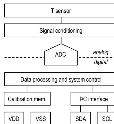
**Figure 1** Functional block diagram of the STSC1.
