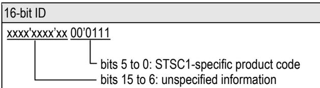
**Table 11** Structure of the 16-bit ID. Bits 15:6 of the ID contain unspecified information (marked as “x”), which may vary from sensor to sensor, while bits 5:0 contain the STSC1-specific product code.
