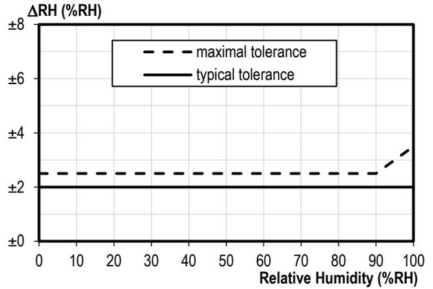
**Figure 3** Tolerance of RH at 25°C for SHT31A
