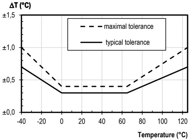
**Figure 8** Temperature tolerance for SHT30A.
