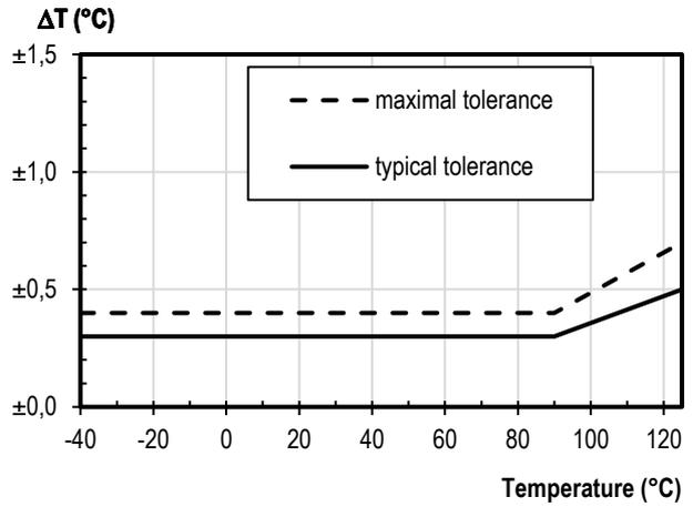
**Figure 9** Temperature tolerance for SHT31A.
