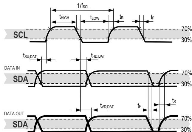
**Figure 12** Timing diagram for digital input/output pads. SDA directions are seen from the sensor. Bold SDA lines are controlled by the sensor, plain SDA lines are controlled by the micro-controller. Note that SDA valid read time is triggered by falling edge of preceding toggle.
