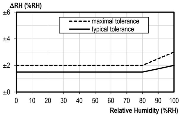
**Figure 4** Tolerance of RH at 25°C for SHT35A.
