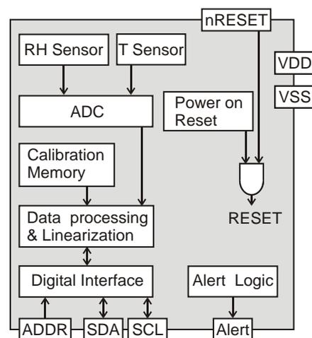
**Figure 1** Functional block diagram of the SHT3xA-DIS. The sensor signals for humidity and temperature are factory calibrated, linearized and compensated for temperature and supply voltage dependencies.
