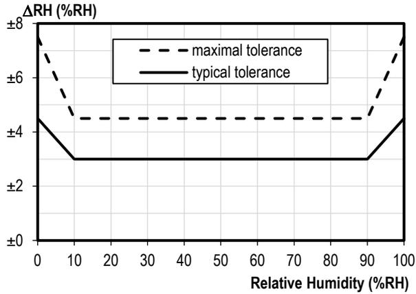
**Figure 2** Tolerance of RH at 25°C for SHT30A
