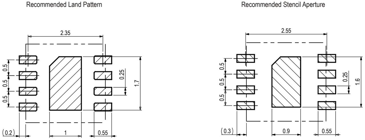
**Figure 15** Recommended metal land pattern (left) and stencil apertures (right) for the SHT3xA-DIS. The dashed lines represent the outer dimension of the DFN package. The PCB pads (left) and stencil apertures (right) are indicated through the shaded areas.
