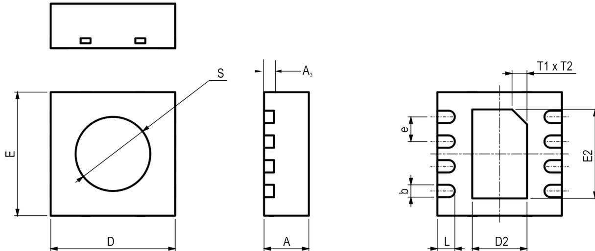
**Figure 14** Dimensional drawing of SHT3xA-DIS sensor package
