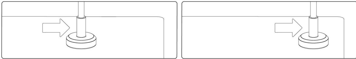
**Detaching the probe** - Tilt the probe foot gently and remove the probe arm. Avoid pulling in the flexible arm!
