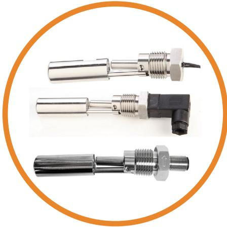
The SSF212 series are horizontally mounted switches that are fitted via a 1/2"NPT thread from the outside of the tank, so does not require access to the inside of the tank.
