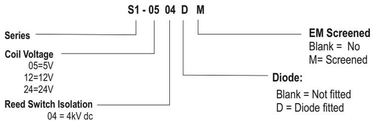
The S1 series is a miniature high voltage single-in-line reed relay for applications where space saving is a prime consideration.
