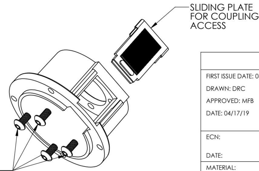
NOTE: USE ENCODER WITH .50 SHAFT EXTENSION FOR PROPER CLEARANCE
