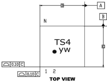
Marking for the 2.0 x 2.0 mm MLPD 8 Lead package:
