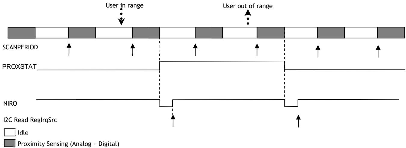
**Figure 19: Proximity Sensing Host Operation (Monitoring Close/Far Events)**
