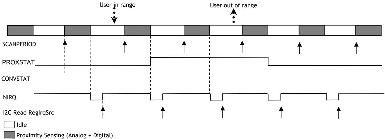
**Figure 20: Proximity Sensing Host Operation (Monitoring Conversion Events)**
