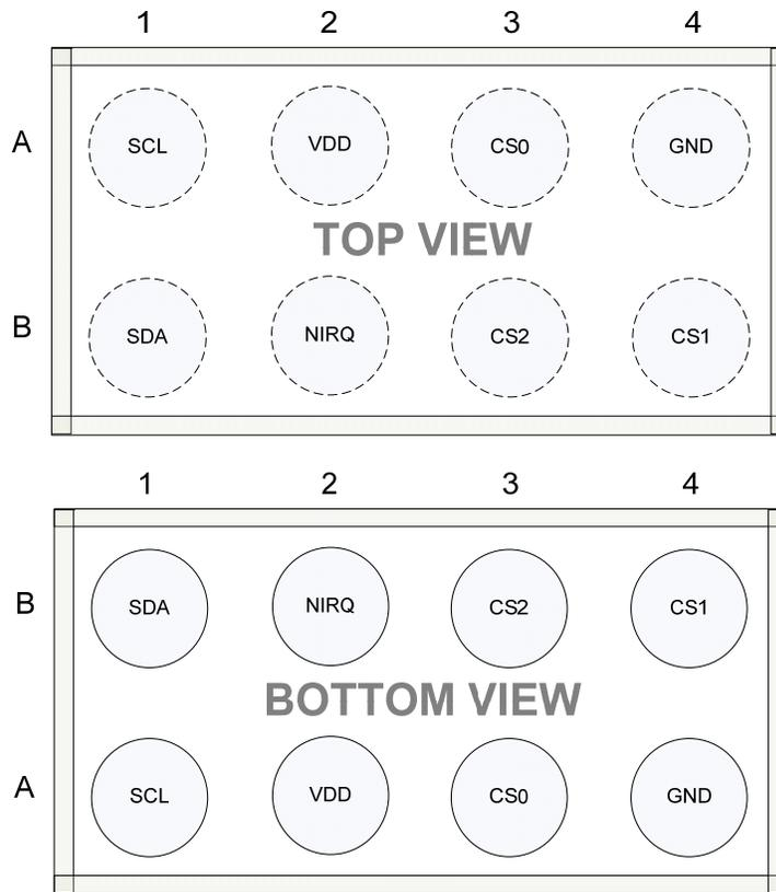
Figure 1: Pin Diagram
