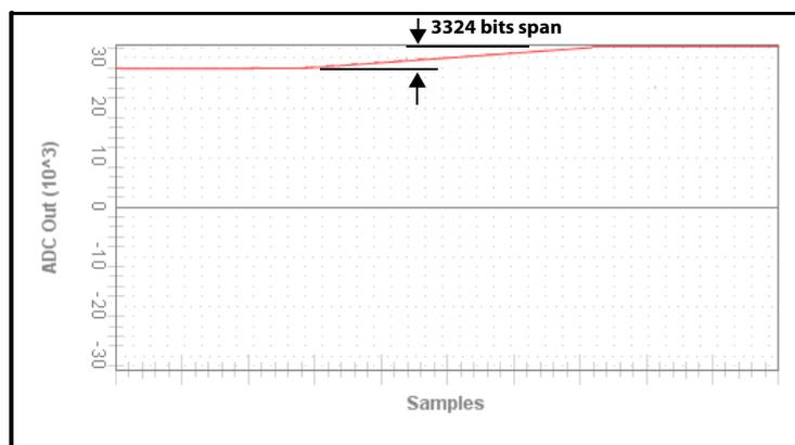
Figure 43. Signal Span Using Rough Gain Setting
