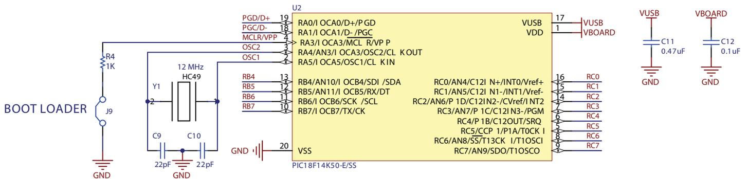
Figure 9. PIC Gateway Schematic
