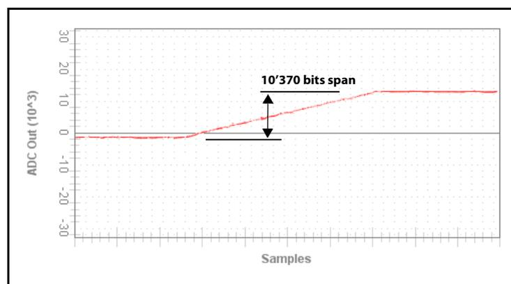
Figure 44. Signal Span Using Zooming Settings
