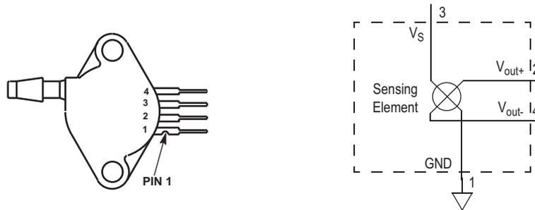
Figure 30. Pressure sensor pin out & equivalent schematic
