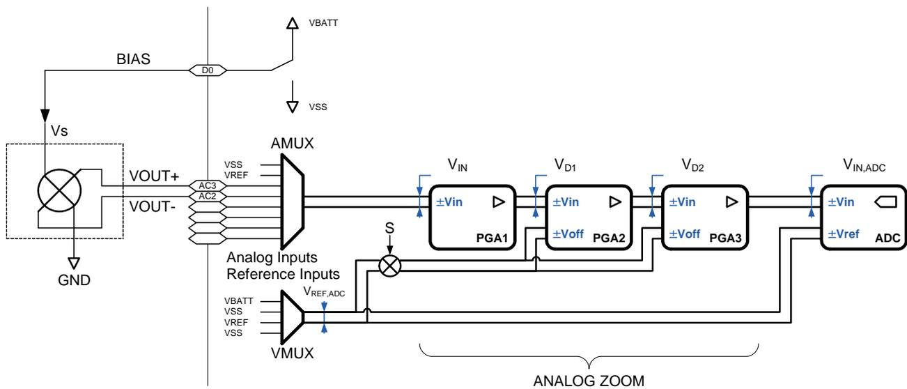
Figure 32. Sensor schematic connection to the SX8724C
