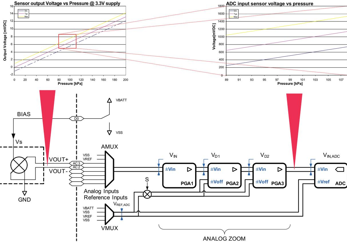
Figure 42. PGA Parameters
