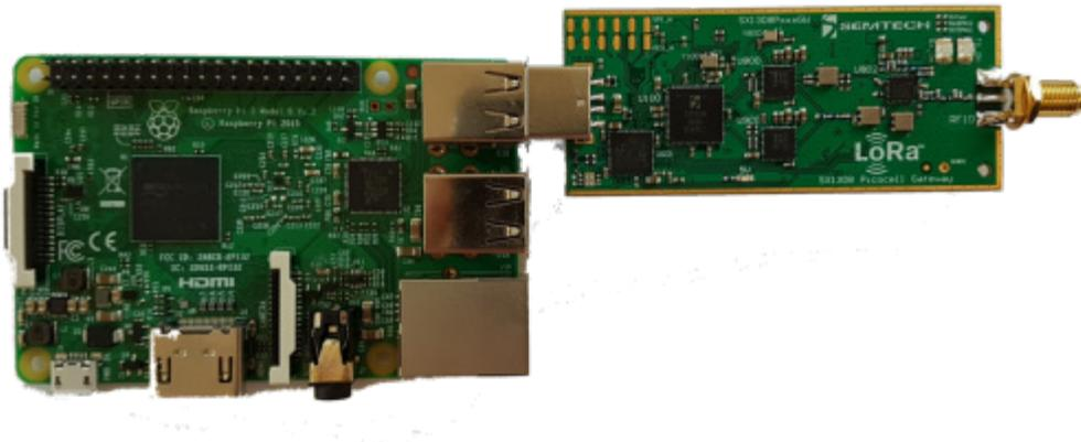
Figure 6: Raspberry Pi and PicoCell GW Connection
