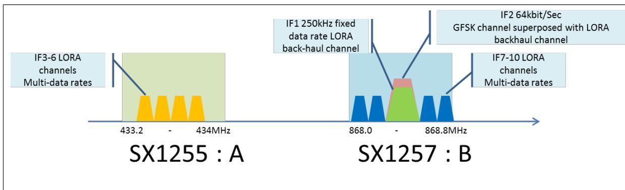
**Figure 11: Radio Spectrum**
