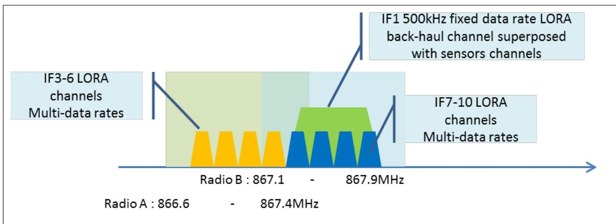
**Figure 10: Radio Spectrum**
