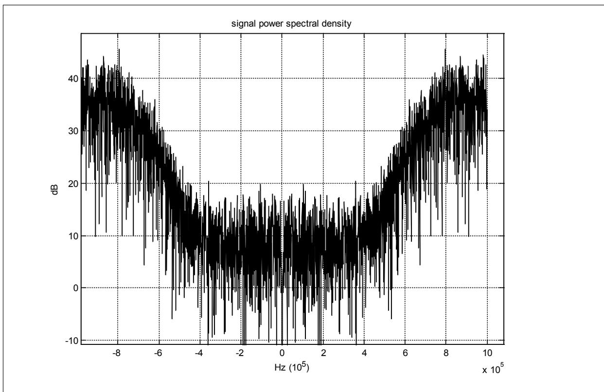
**Figure 8: SX1255/57 Digital I/Q Power Spectral Density**
