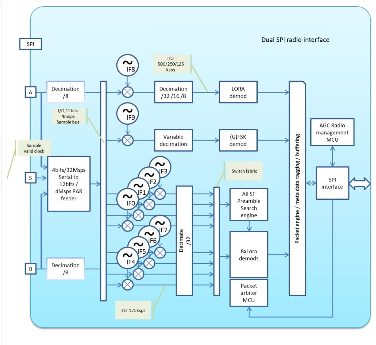
**Figure 6: SX1308 Digital Baseband Chip Block Diagram**
