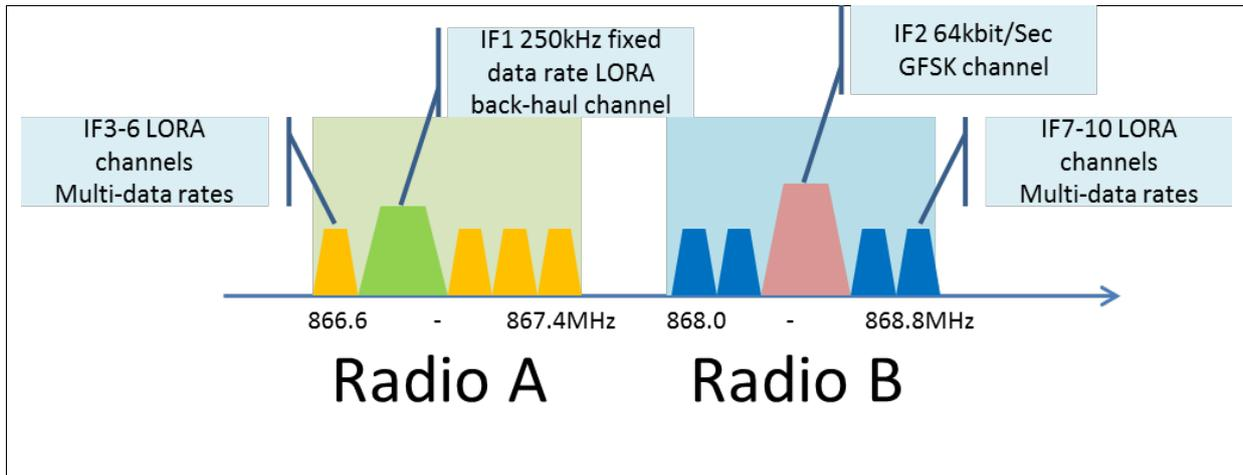
**Figure 9: Radio Spectrum**
