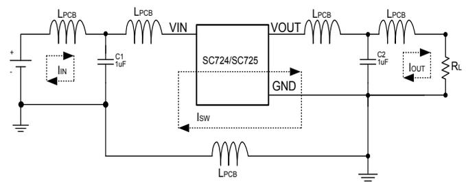
**Figure 1 - PCB Circuit with Equivalent Parasitic Inductance**
