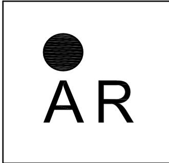
Marking for the 0.76 x 0.76 mm CSP 4 Lead Package :
