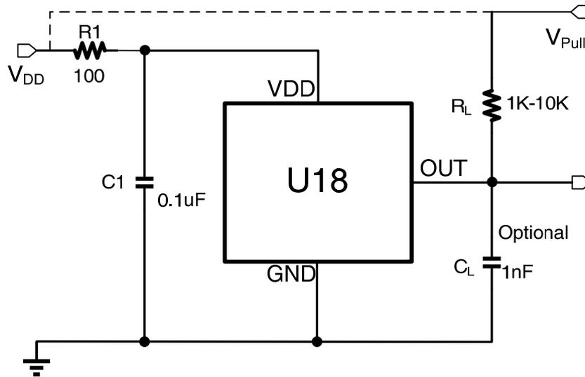
The U18 contains an on-chip voltage regulator and can operate over a wide supply voltage range. In applications that operate the device from an unregulated power supply, transient protection must be added externally. For applications using a regulated line, EMI/RFI protection may still be required. R1 is for improved CI performance, and could be 100 or 200  $\Omega$  typically.
