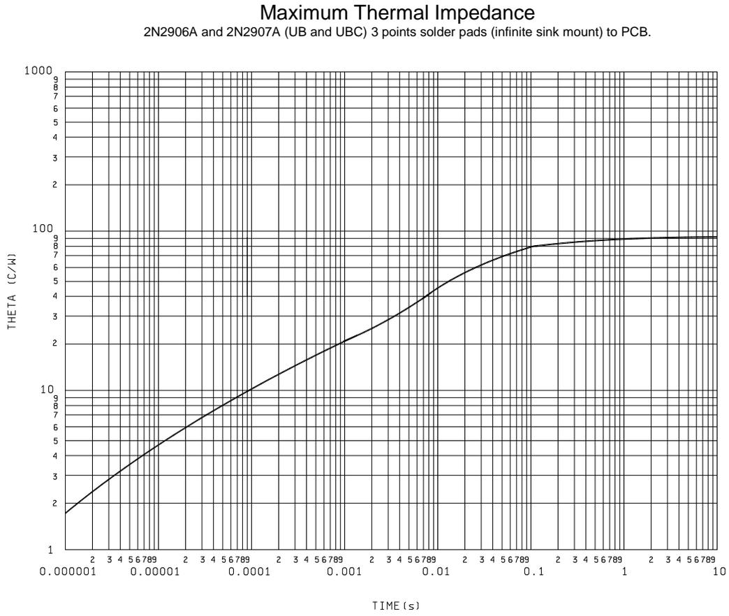
FIGURE 15. Thermal impedance graph ( $R_{\theta JSP(IS)}$ ) for 2N906A and 2N2907A (UB, UBC, UBN, and UBCN).
