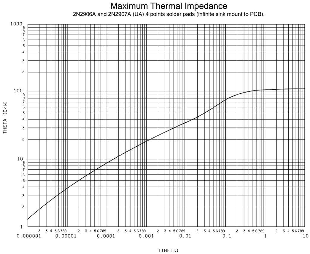
FIGURE 13. Thermal impedance graph ( $R_{\theta JSP(IS)}$ ) for 2N906A and 2N2907A (UA).
