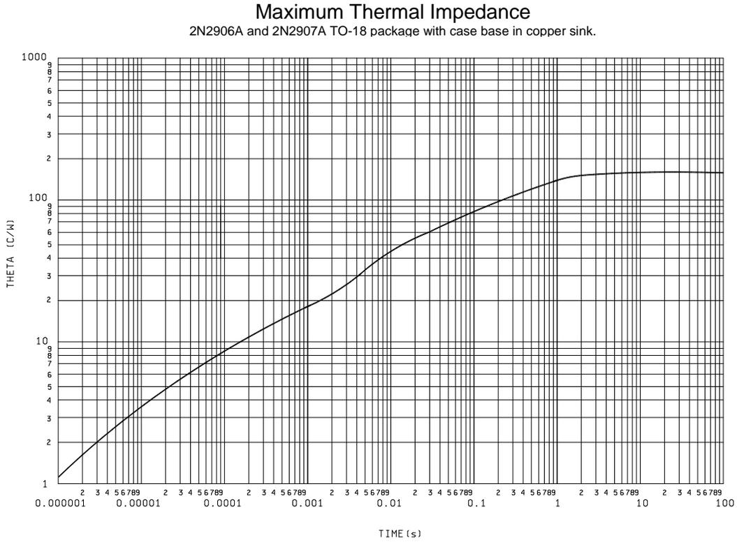
FIGURE 12. Thermal impedance graph ( $R_{\theta JC}$ ) for 2N2906A, 2N2906AL, 2N2907A, and 2N2907AL (TO-18).
