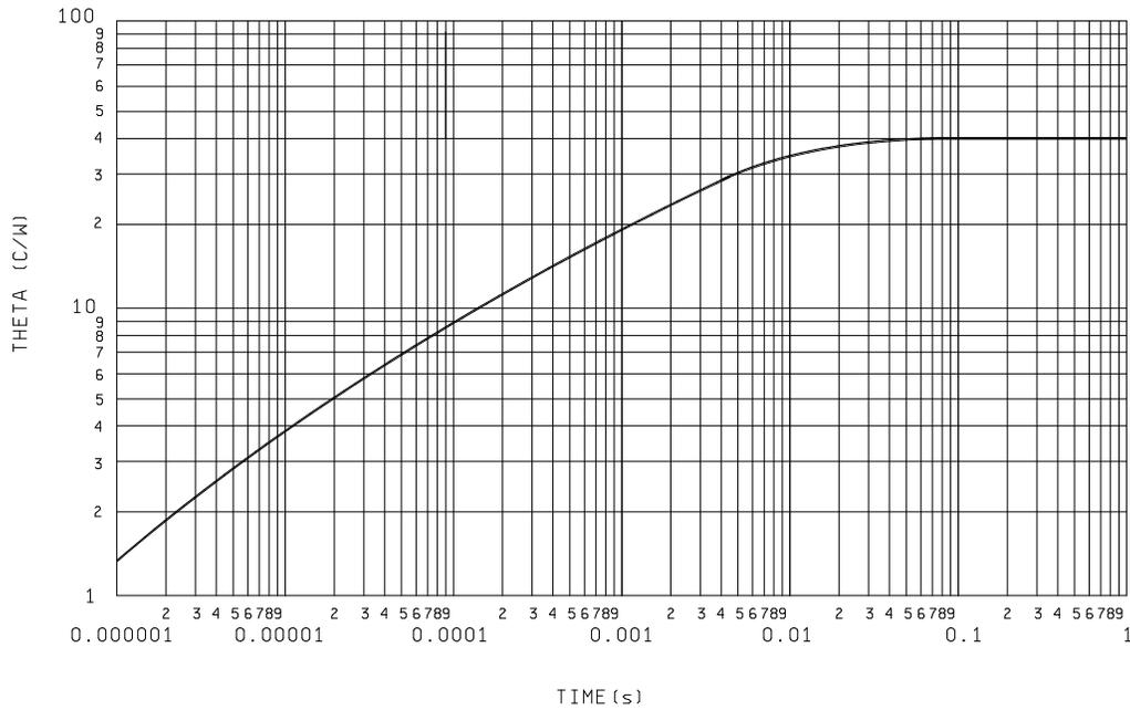
FIGURE 14. Thermal impedance graph ( $R_{\theta JSP(AM)}$ ) for 2N906A and 2N2907A (UA).
