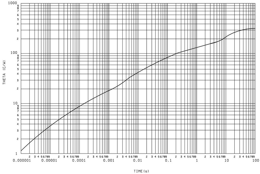
FIGURE 11. Thermal impedance graph ( $R_{\theta JA}$ ) for 2N2906A, 2N2906AL, 2N2907A, and 2N2907AL (TO-18).
