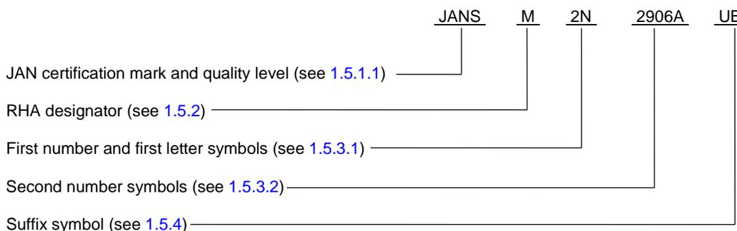
\* 6.6.2 Unencapsulated devices. The PINs for un-encapsulated devices are constructed using the following form.
